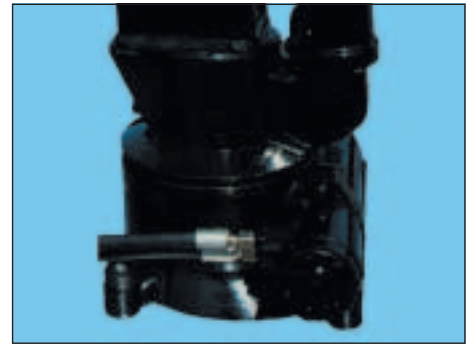
The O-ring-sealed slewing housing of cast steel with an encased worm gear prevents water and dirt from entering.
